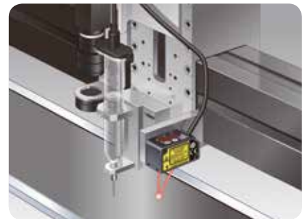
Controlling the dispenser head height
